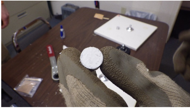
Figure 22 Paint Supplier-Dollie separated from glue bond
