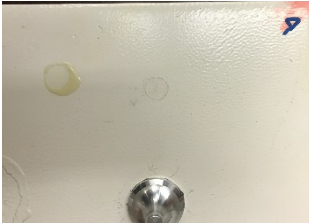
Figure 23 Sample after Paint Supplier Pull Test
