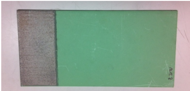
Figure 3 Navy primer on steel, back side of non-skid
